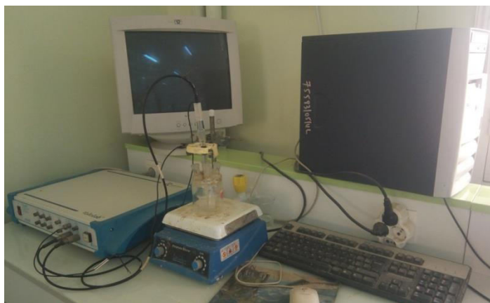
Figure 2: electrochemical assembly with three electrodes
