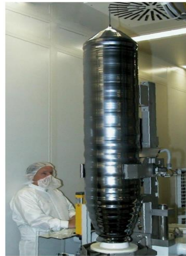
Fig. II. 3 Silicon crystal with a diameter of 300 mm and a weight exceeding 250 kg, grown by the Cz method.
