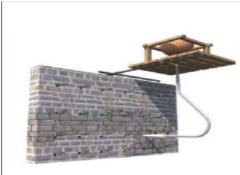
Figure 34 : Cimentation par injection sous pression, (source: Z.Damene, M.S.Goual, T. Bourzeg, Y.Daikh , jan 2015, Study of pathological cases in the district of Zegague Elhadjaj, Journal of fundamental and applied sciences , p 72).
