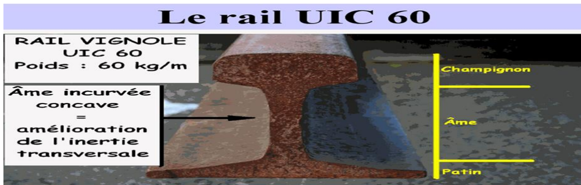
Figure VI. 8: le rail UIC 60
