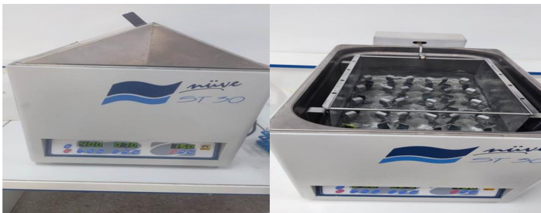
Figure II.3 : Bain thermostaté agitant.
