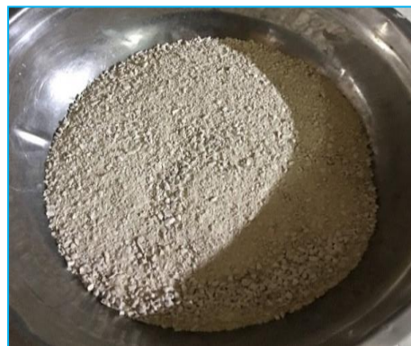
Crushing limestone sand (CS)
