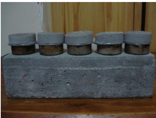
Fig2.failure mode of repair mortars: (a) Control mortar,(b)M00100,(c)Ready-mixed mortar.
