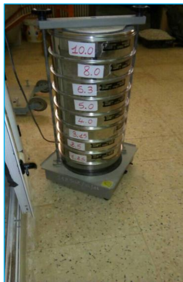
Figure II.3. Sieve analysis of gravel (3/8).
