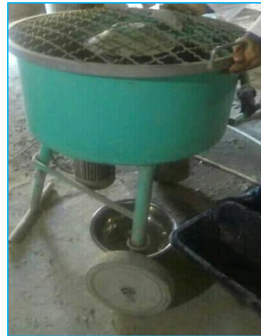
Concrete mixer with a 60 litres of capacity.
