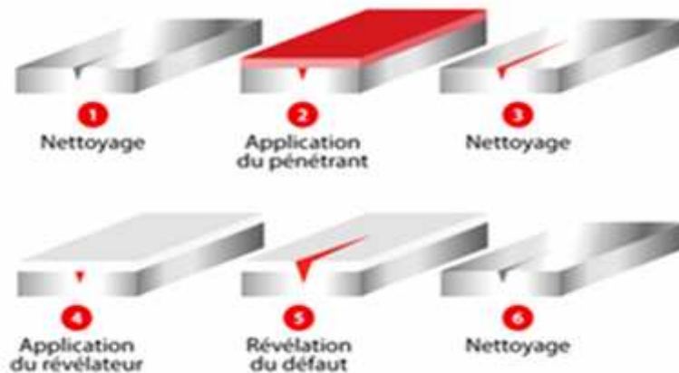
Figure I.3- Principe du ressuage .
