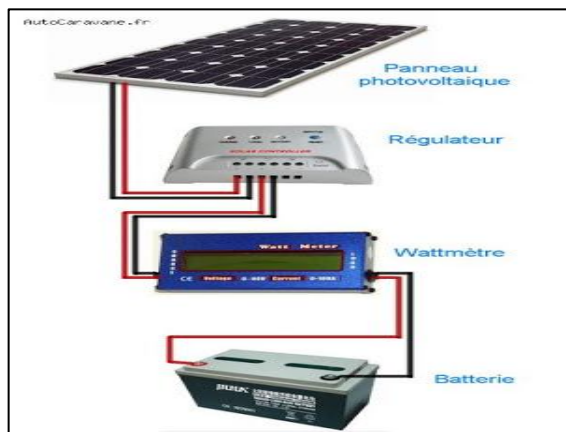
Figure 96: installation Dun Panneaux photovoltaïque
