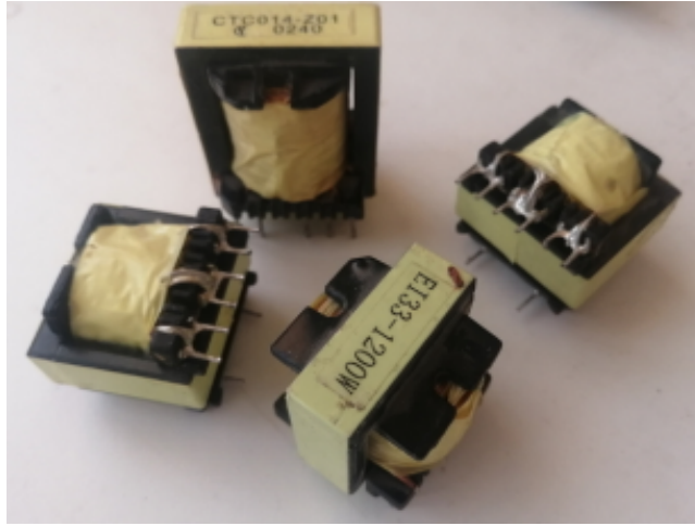
Figure 1.4: Example of a set of transformers used for galvanic isolation in DC-DC converters.
