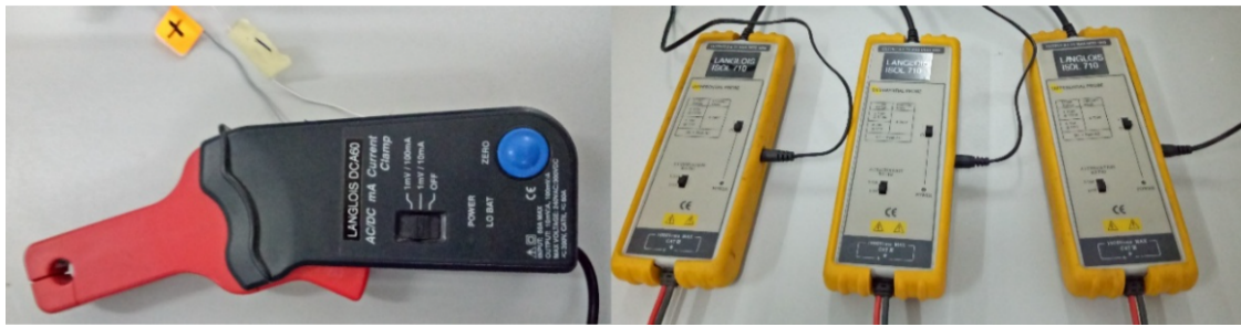
Figure 3.8: Current and voltage measurement sensors
