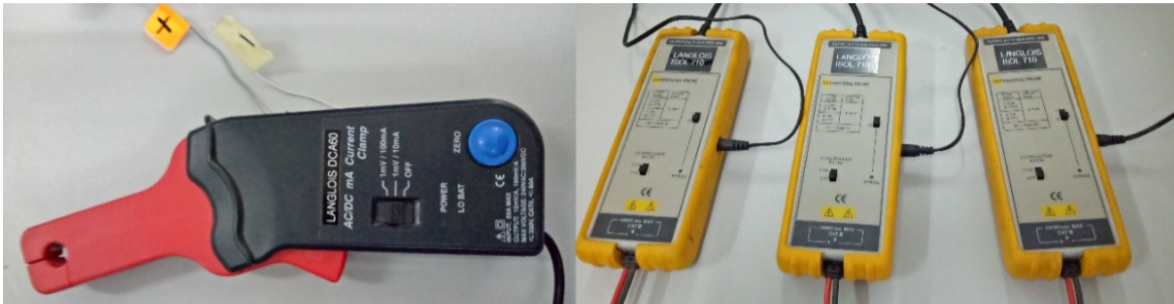
Figure 3.12: Current and voltage measurement sensors.
