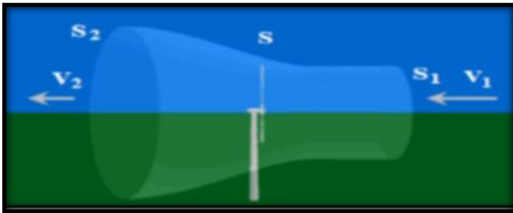
Fig 17 : Current tube around a wind turbine [41].
