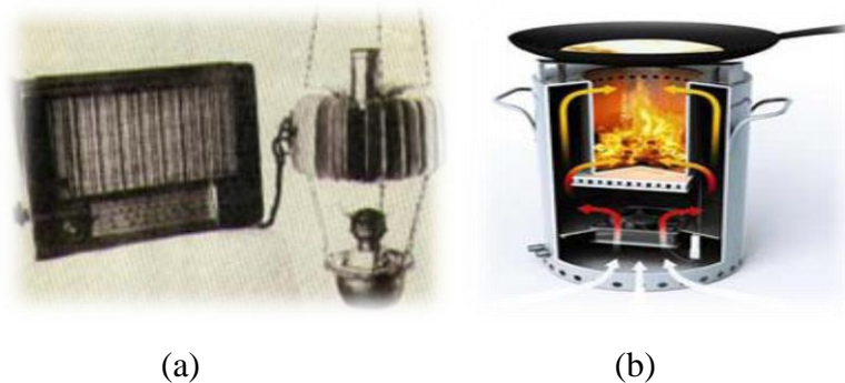
Figure I. 7 : Radio powered by thermoelectric module using the heat of a kerosene lamp (a), wood burning oven with integrated thermoelectric module for the production of electricity (Philips Research) (b).
