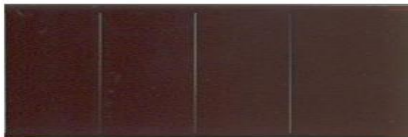
Figure I - 7 : Cellule photovoltaïque amorphe [7]
