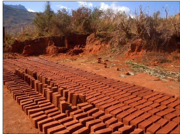
Figure II.16: fabrication d'adobe source : http://www.africavernaculararchitecture.com
