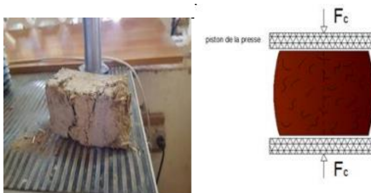
Figure I.20 : Essai de compression
