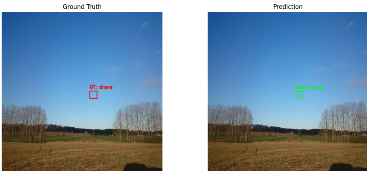
Figure 3.5: Ground Truth Bounding Box and Predicted Bounding Box of a Drone
